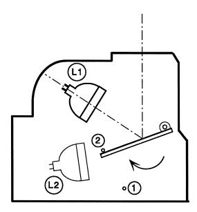
In the Service Software TL-4575 there is an option in the menu "Lamp toggle" to check the MIRROR FUNCTION and change the "lamp on" option. For the correct function in the projector, set the MIRROR to position 1 when Lamp 1 is active, or reset the projector.
